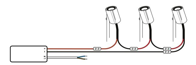
TYPICAL WIRING. NOTE SERIES CONNECTION - INTO POSITIVE, OUT OF NEGATIVE INTO POSITIVE ETC. Easy connection boards are available as an alternative.
